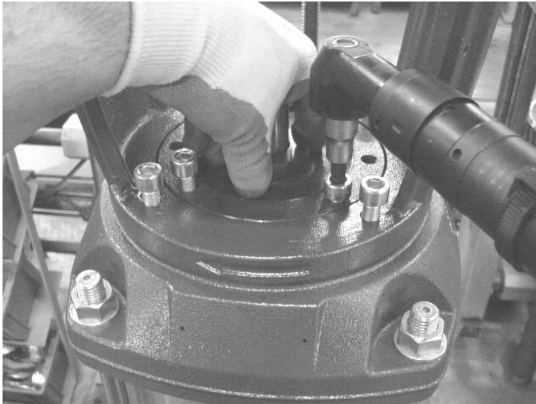
Seal housing disc installation Cross-tightening required.
