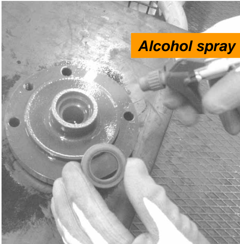
Replacement of stationary part of mechanical seal
