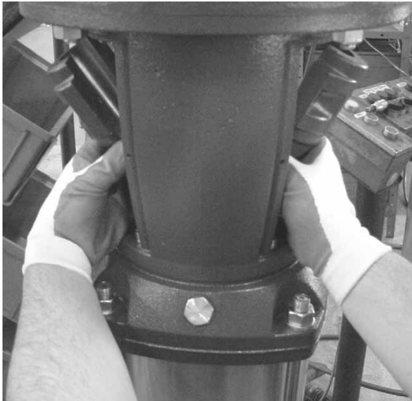
Removal of coupling and pin
