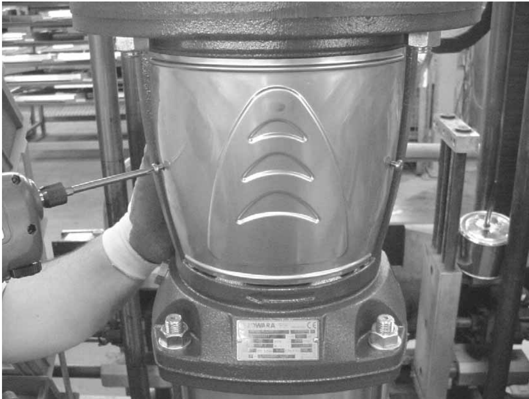
Coupling guard installation
